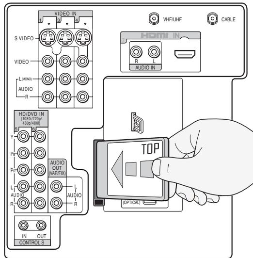
**CAUTION:** Inserting the CableCARD incorrectly may result in permanent damage to the card and the TV.
