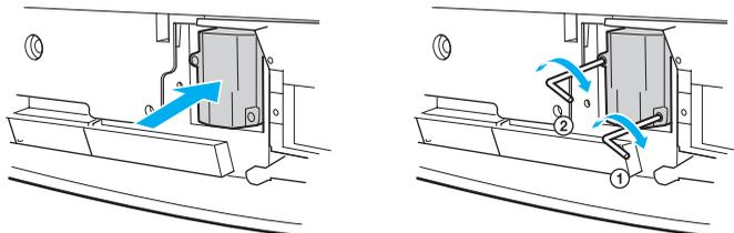
Place back the lamp cover, then tighten the screw.
