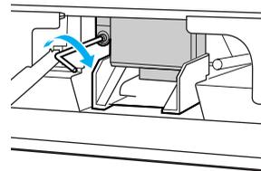
Push the cover back on. Make sure that the hole on the cover aligns with the hole on the unit. Reattach the lamp cover by tightening the screw.
