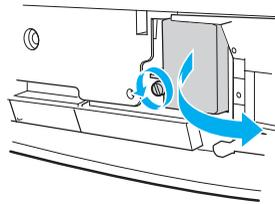
Loosen the two screws that hold the lamp, then pull out the lamp.
