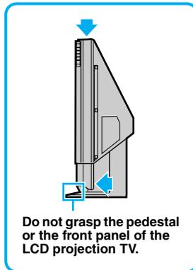
When moving the LCD projection TV, place one hand in the hole on the lower portion of the TV while grasping the top with the other hand, as shown in the illustration below.
