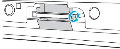
Remove the screw from the lamp cover. Pull down the cover toward you.
