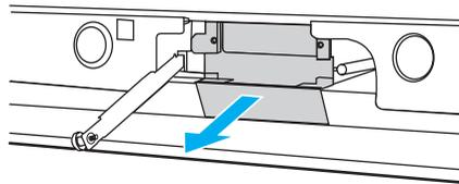
Unscrew the lamp and pull out the lamp horizontally.
