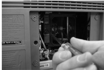
4 Separate the Lamp from the engine by holding the handle and pulling it out.
