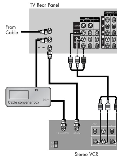
Caution: If you want to record one channel while watching another channel, a splitter (not included) must be added between the cable and "ANT 1 IN". One output of the splitter goes to "ANT 1 OUT" and the second output is connected to IN on the cable converter box.
