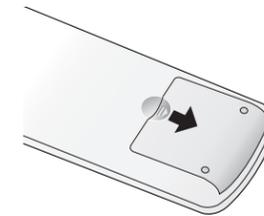
2 Install two AAA size batteries. Make sure to match the "+" and "-" ends of the batteries with the diagram inside the compartment.
