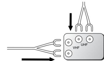
2 Plug the combiner into the "ANT 1 IN" terminal on the rear panel.
