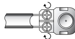
2 Plug the adaptor into the "ANT 1 IN" terminal on the rear panel.
