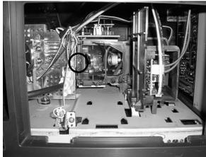
5 Separate the Lamp from the engine by holding the handle and pulling it out.
