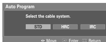
5 Press the ENTER button to start the auto program. The TV begins memorizing all available stations. Press the ENTER button at any time to interrupt the memorization process.
