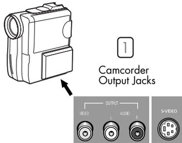
2 Connect a set of audio cables between the AUDIO IN jacks on the TV and the AUDIO output jacks on the camcorder. If you have a mono Camcorder, connect L(mono) to the Camcorder audio out using only one audio cable.
