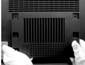
3 Remove the Lamp cover duct holding the tab and pulling it out.
