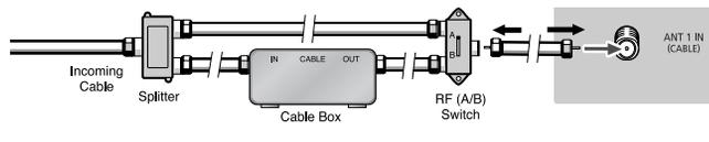
After you've made this connection, set the A/B switch to the "A" position for normal viewing. Set the A/B switch to the "B" position to view scrambled channels. (When you set the A/B switch to "B", you will need to tune your Set-Top Box to the Cable box's output channel, which is usually channel 3 or 4.)
