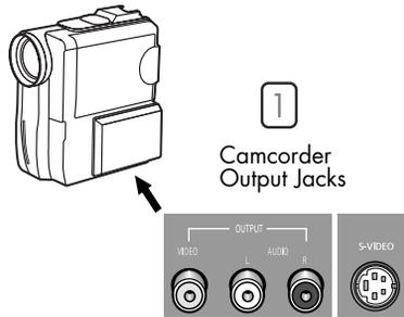
**2** Connect a video or S-Video cable between the VIDEO IN (or S-VIDEO IN) jack on the TV and the VIDEO (or S-VIDEO) output jack on the Camcorder. The audio-video cables shown here are usually included with a Camcorder. (If not, check your local electronics store.) If your Camcorder is stereo, you need to connect a set of two cables.
