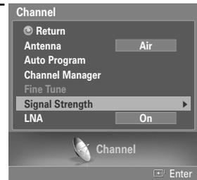
If the signal strength meter indicates that the signal is weak, physically adjust your antenna to increase the signal strength. Continue to adjust the antenna until you find the best position with the strongest signal.
