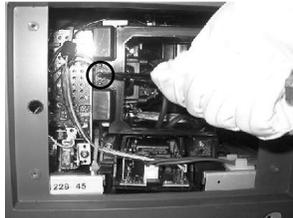
4 Separate the Lamp from the engine by holding the handle and pulling it out.
