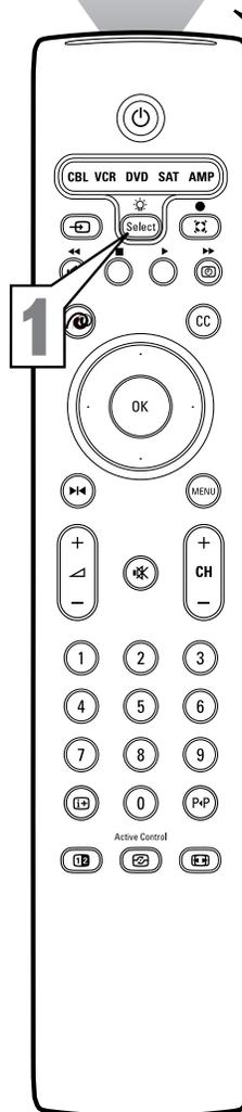
Point the front of the remote toward the front of the accessory device, then press the necessary buttons to perform the functions you desire. Refer to pages 27 to see the functions of the buttons in the respective accessory modes.
