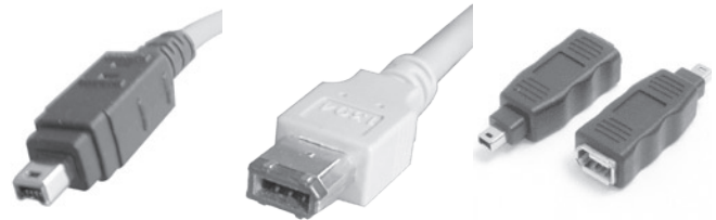
4-pin connector 6-pin connector 6-pin-to-4-pin adapter
