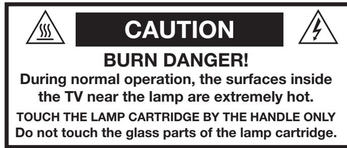
**CAUTION:** If the television is on, press **POWER** to turn it off. Unplug the television and allow it to cool for at least one hour before attempting to replace the lamp cartridge.
