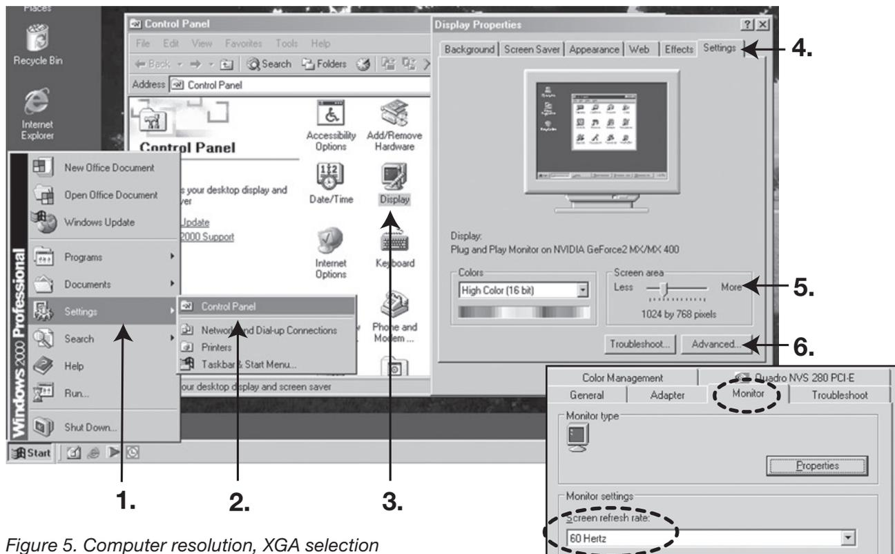
Figure 5. Computer resolution, XGA selection
