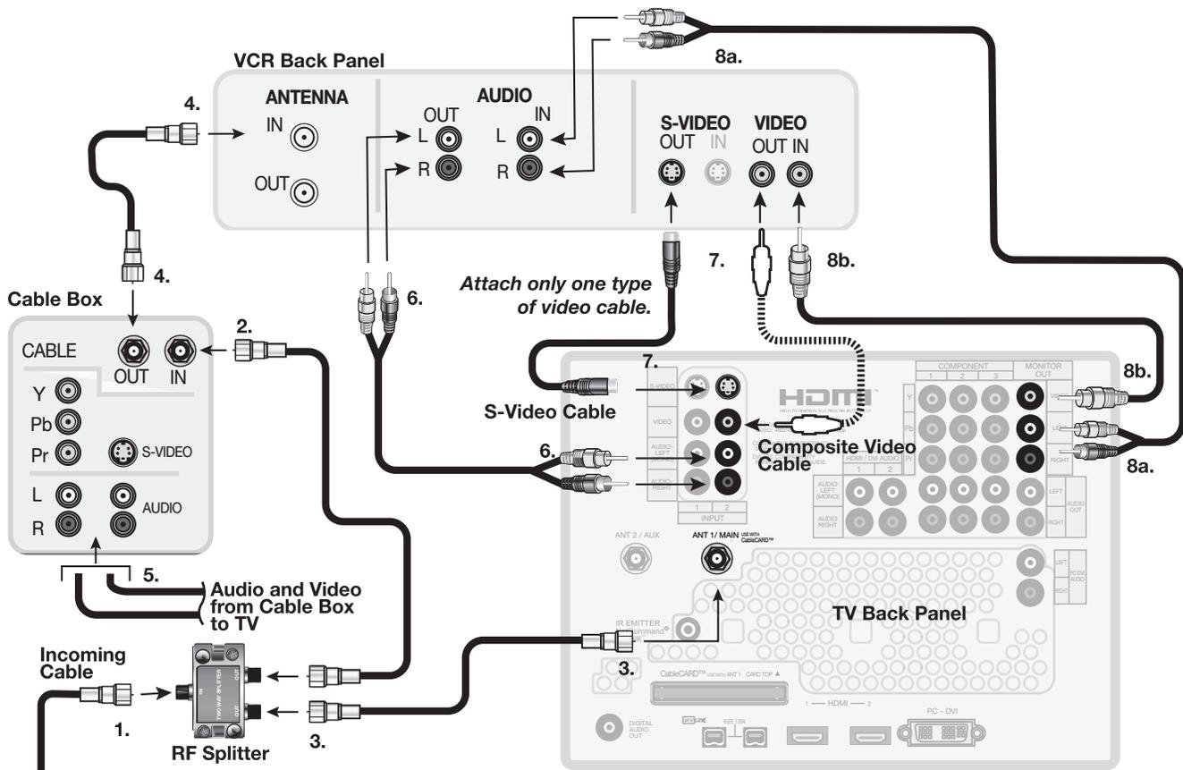
Figure 7. Connecting a VCR to a cable box
