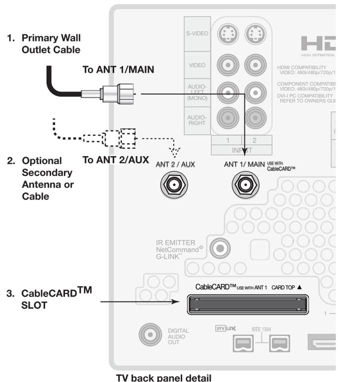
Figure 3. Wall Outlet Cable
