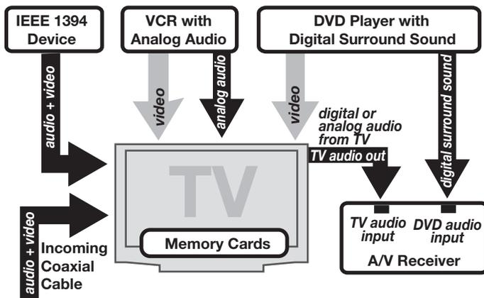
Figure 14. Overview of A/V receiver connections described
