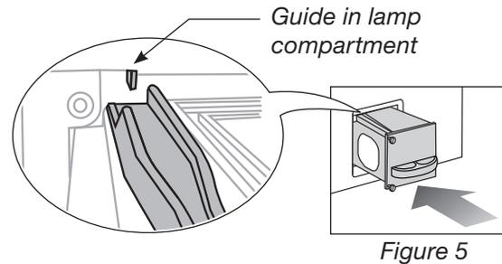
2. With either your fingers or the screwdriver, gently tighten the two shiny screws. If using a screwdriver, use only two fingers for final tightening. **AVOID OVERTIGHTENING!**
