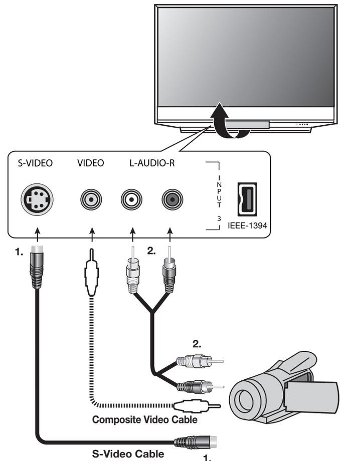
Figure 13. Analog connections for a camcorder
