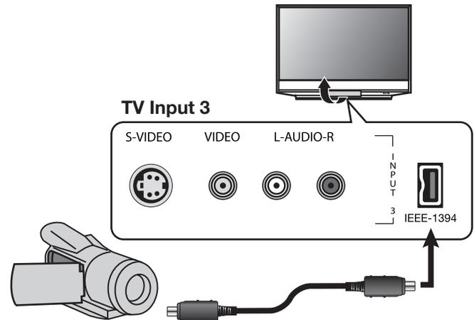
You can connect an IEEE 1394 camcorder with an IEEE 1394 cable or with analog audio/video cables. In either case, test using the TV's remote control to operate the camcorder via the IEEE 1394 cable.
