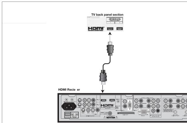
Figure 11. Connecting an HDMI Device
