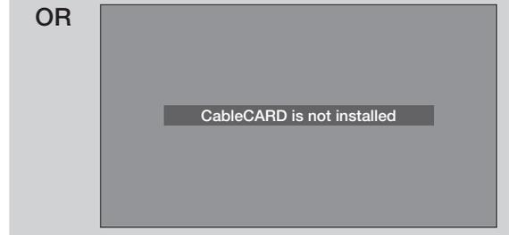
After the CableCARD is installed, wait until the second screen below appears. The third screen below will appear if a channel is not authorized for viewing. Press the **EXIT** button to exit the second screen.
