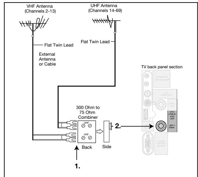
Figure 4. Connecting separate UHF and VHF Antennas
